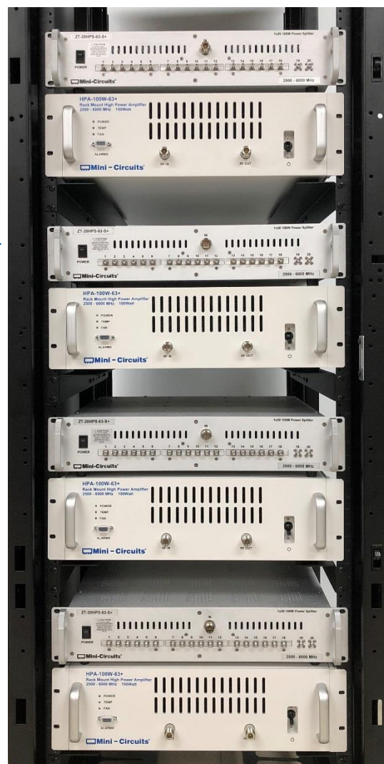
Figure 2 Rack Setup for HTOL System
